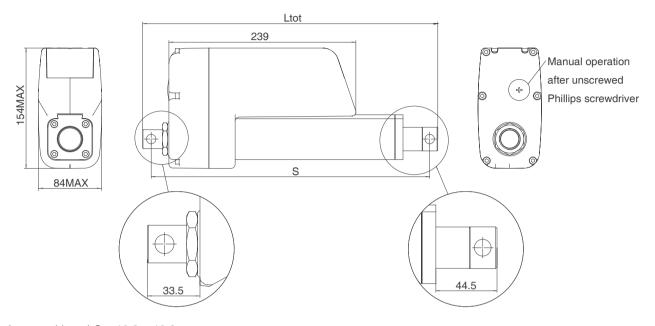
Ltot: total lengthS + 10.9 + 10.9 S Installation distance: 255 + stroke
